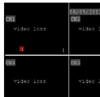
Main Viewing Screen Showing No HDD in DVR
