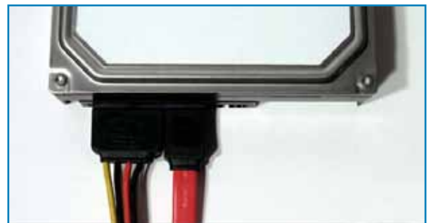
Hard Drive - Remove/Connect Cables
